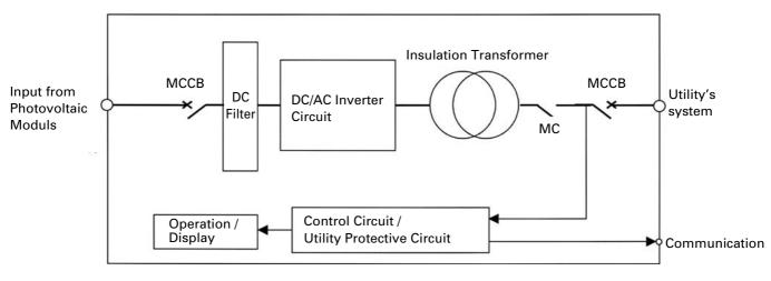
Fig. 2: Block Diagram of the "SANUPS P83A"
